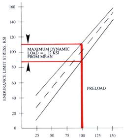
Modified Goodman diagrams help designers predict fastener performance. The broken diagonal line depicts the mean of the alternating load for a screw with a 90% probability of enduring 10 million cycles. The diagonal solid lines show that the maximum deviation of dynamic load from the mean stress is :t12 ksi when the screw is pre-loaded to 100 ksi.
