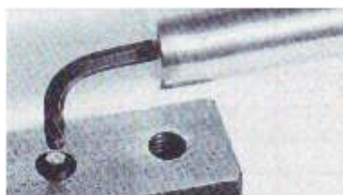
Twisted to about 270^\circ , the key shears off clean. Note the extension bar illustrated for test purposes only.
