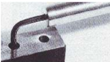
A 5/64 " UNBRAKO key will twist up to 180^\circ without weakening.
